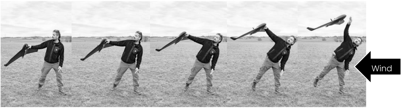
Figure 4-9 Nose launch procedure
