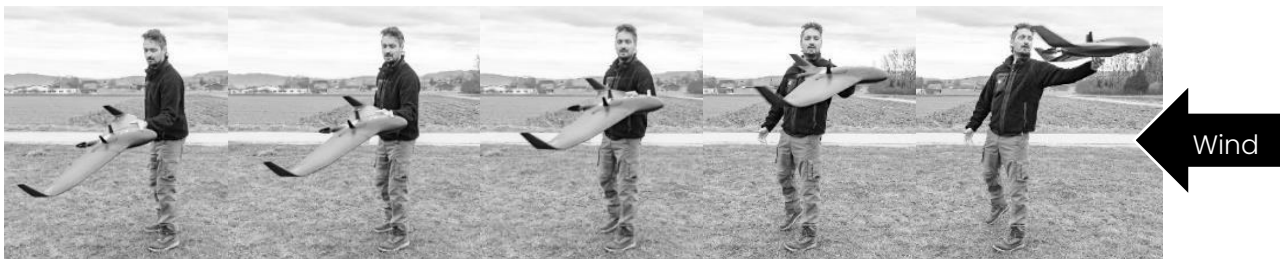
Figure 4-7 Typical hand launch procedure
