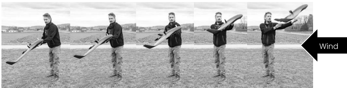
Figure 4-8 Two hand launch procedure
