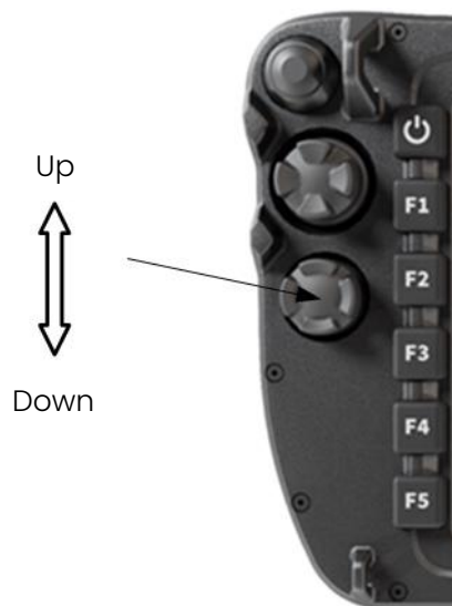
Figure 4-35 Fast climb/descent altitude control
