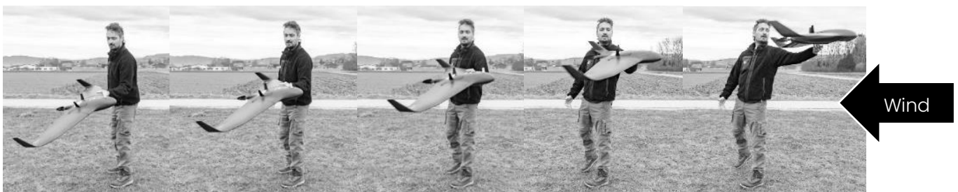
Figure 4-6 Typical hand launch procedure
